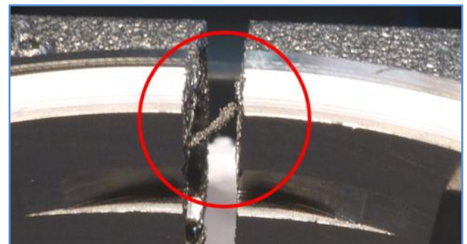
Cracked connection rod [1]
