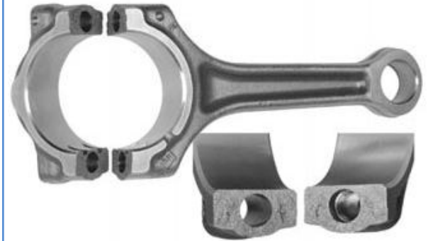
Cracked connection rod [1]
